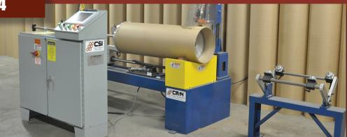
Western Container, from Beloit, Wisconsin, has launched a new addition to their production capabilities. The CM-14 has recently been added to the manufacturing line to meet the needs of large precision re-cutting. The CM-14 is a heavy-duty automatic core cutter designed to cut cores with large internal diameters with ease and speed.
